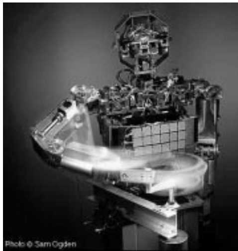
Figure 1-2: COG is a humanoid robot with upper torso, arms and head. The arms use series elastic actuators for each of its six degrees of freedom. Here COG is turning a crank using a dynamic oscillating controller.
