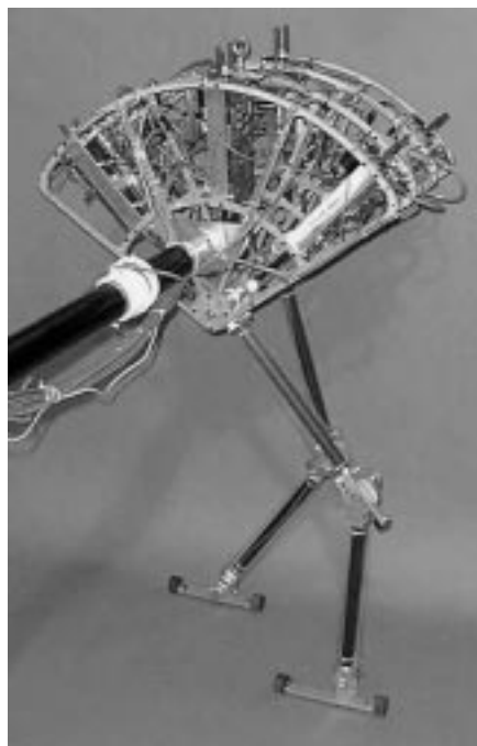
Figure 1-3: Spring Flamingo is a planar bipedal walking robot. It uses series elastic actuators to actuate its six joints. Its top walking speed is 1 m/s.
