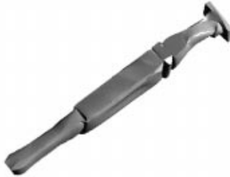
Figure 6: The razor is scanned and reconstructed into a BRep solid model.
