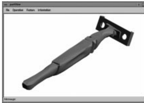
Figure 7: The complex sculptured razor CAD model is unioned with a standard head.
