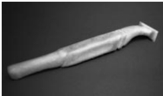
Figure 5: One of the razors carved by a designer. Starting from the rapid prototyped model, he used simple hand tools to create the complex shape.
