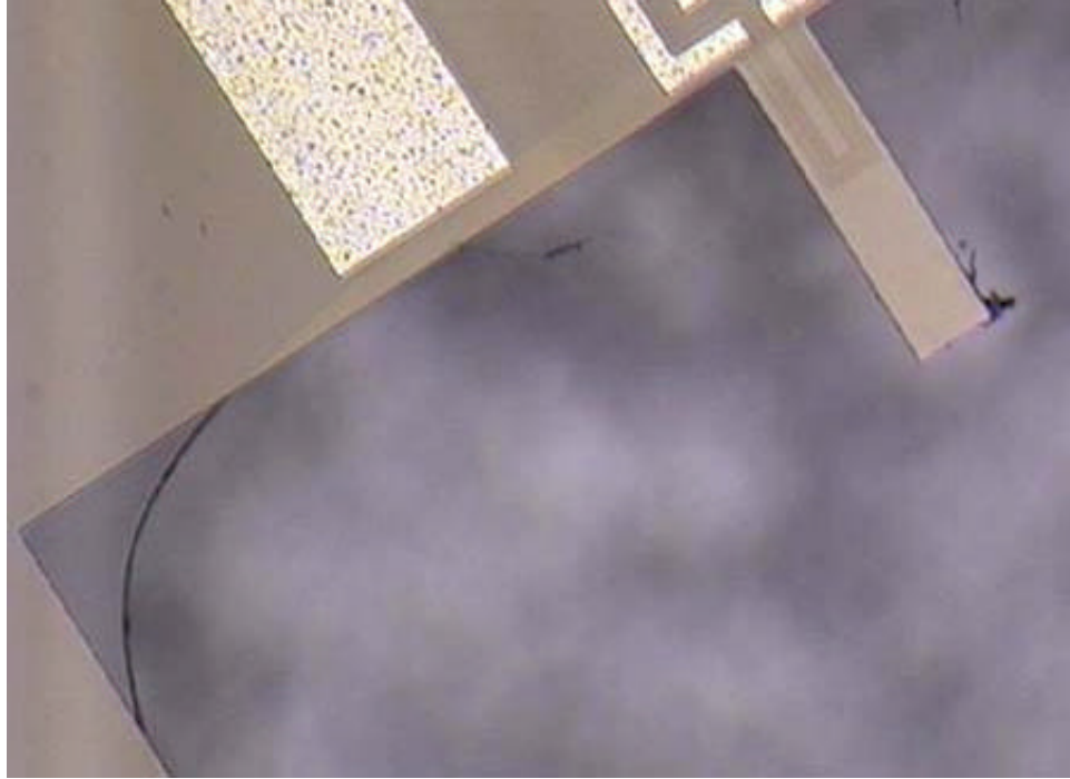
Figure 8 --- Footing and underetch from STS. The curved corner at the left is residual silicon, while the light region which extends the curve towards the cantilever, shows where only the top layer of silicon remains. Also note aluminum oxide residue attached to end of cantilever.
