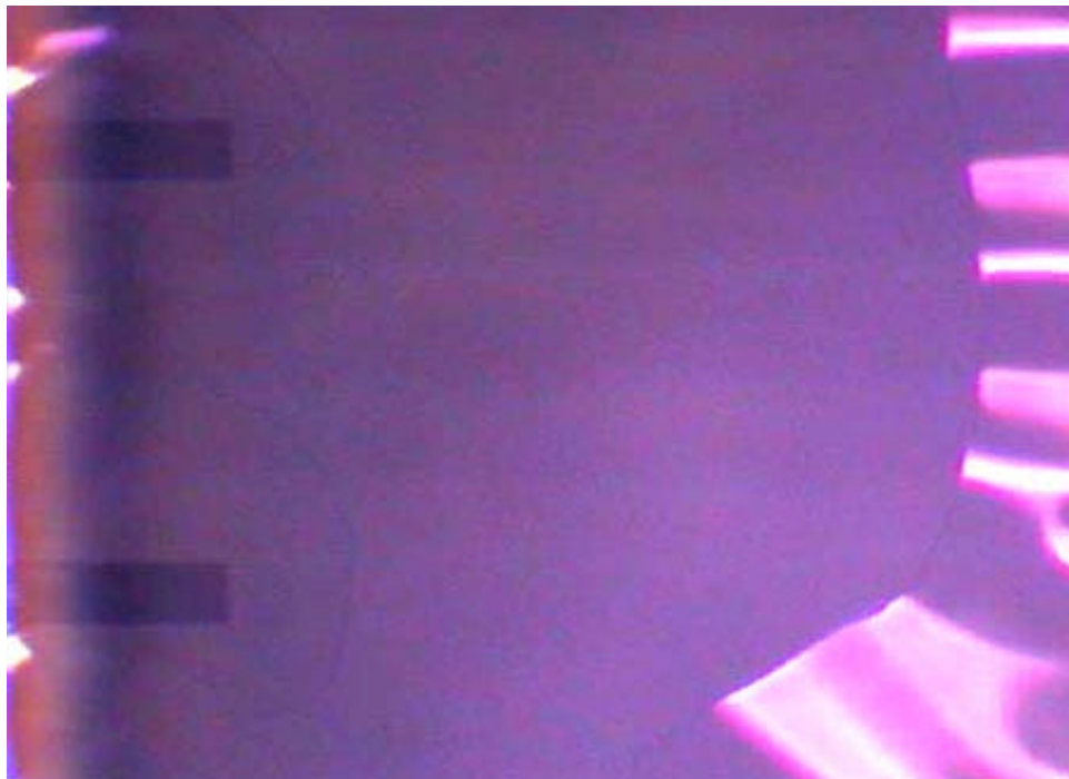
Figure 9 --- Suction damage. The membrane layer was shattered when the asher vacuum chuck picked up the wafer. In this example, the cantilevers at left actually reinforced the layer, and islands of the membrane remained around them.
