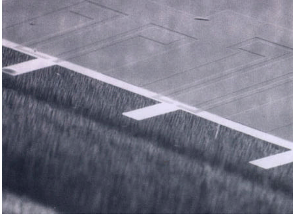
Figure 10 --- Completed piezoresistive microcantilevers. This SEM shows typical cantilevers, together with the aluminum contact pads. Note the undercutting of the cantilever silicon layer (white strip). This device was used in the resonant frequency tests. The leftmost cantilever has adhesive remaining on it.
