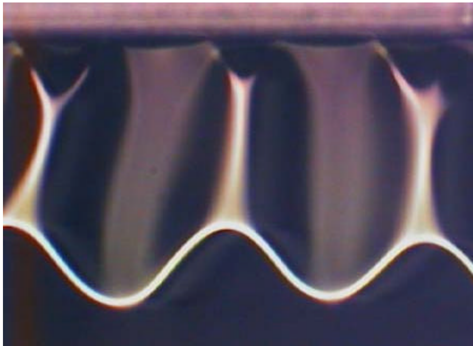
Figure 5 --- Highly buckled SOI oxide layer. A test wafer had PI removed prior to the oxide etch, so oxide is unrestrained from buckling. Note sharp peak of buckled membrane.
