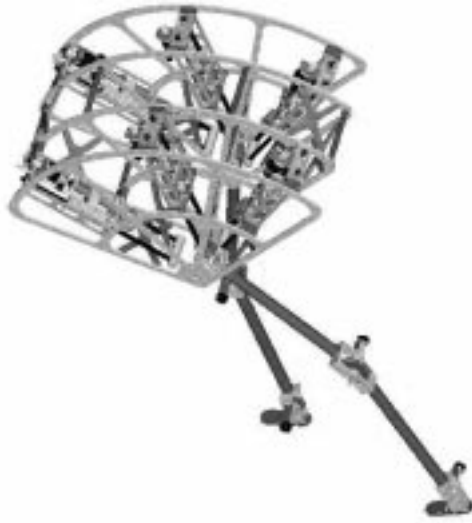
Figure 1: Spring Flamingo: A 7-link planar bipedal robot currently under construction.
