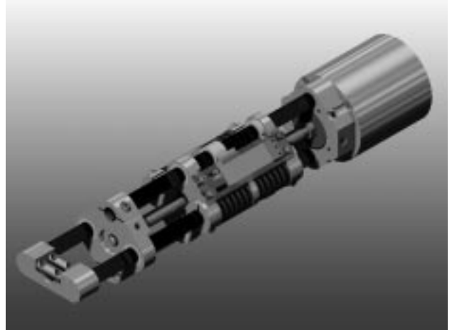
Fig. 1. The prototype actuator has a brushless DC motor rigidly connected to a ballscrew which drives the linear motion. The ballscrew nut is coupled to the output through four die compression springs. The spring compression is measured with a linear potentiometer. The actuator can output over 1350 N and move at 25 cm/second.
