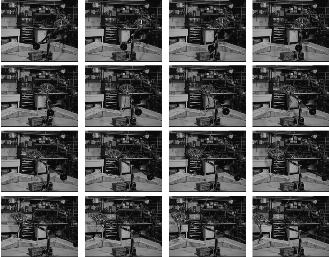
Figure 4-9: REAL Video frames of Spring Flamingo walking over rolling terrain with 15^\circ upslopes and downslopes. Frames proceed left to right with 0.5 seconds between frames.
