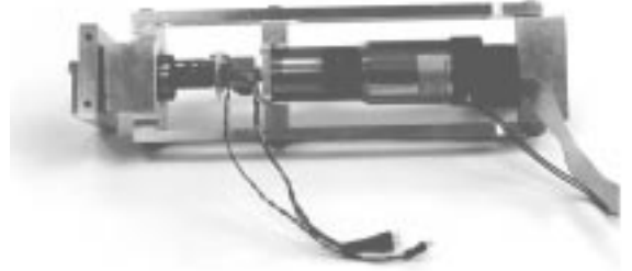
Figure 11: Photograph of Experimental Series-Elastic Actuator
