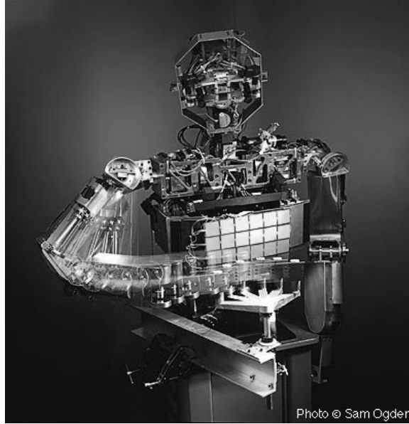
Figure 4-17: [Picture of Cog turning a crank] Picture of Cog turning a crank. The robot is using two shoulder joints and two elbow joints to create the motion of the crank.
