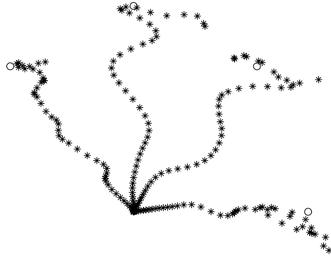
Figure 3-29: The simulated trajectory in the HFF. The trajectory is distorted significantly corresponding to the forces.
